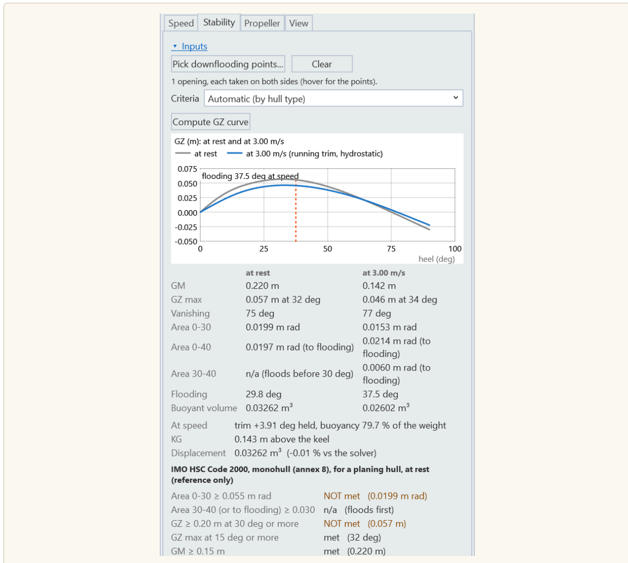
Figure 6 The Stability sub-tab: a downflooding point, the GZ curves at rest (grey) and at the selected speed (blue) with the flooding angle marked, and their measures side by side.
